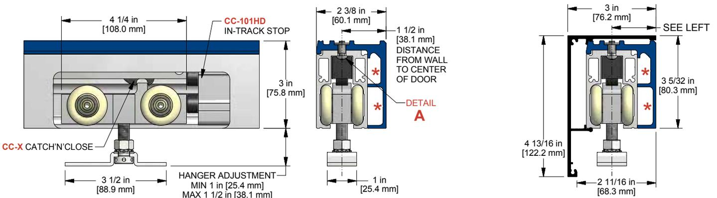
[CC-902 Side Mount Bracket illustrated as solid blue profile. Supplied in continuous lengths.]
