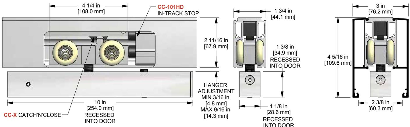
[Optional **CC-940** Snap-On Fascia illustrated as solid **black** profile. Can be used on both sides of the track or one side only]
