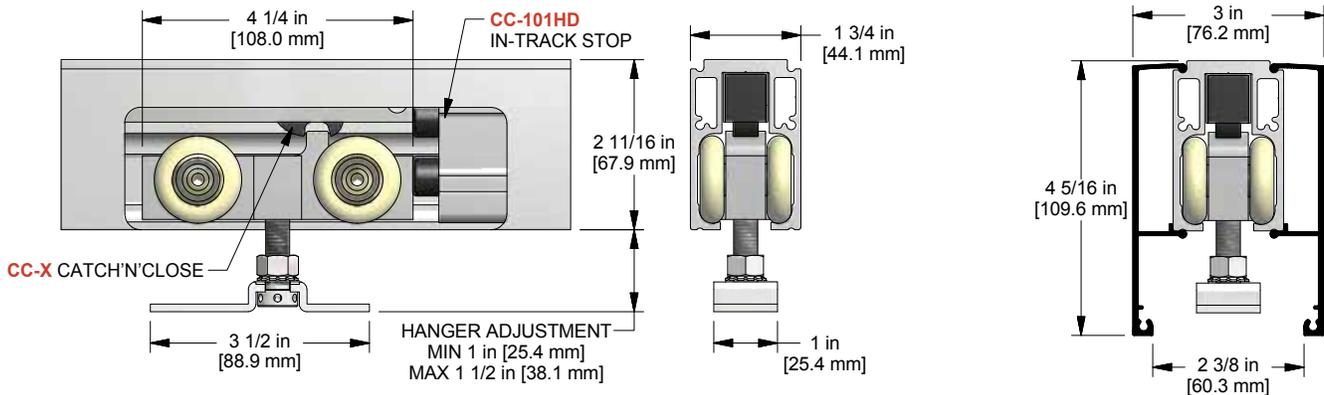
[Optional **CC-940** Snap-On Fascia illustrated as solid **black** profile. Can be used on both sides of the track or one side only]
