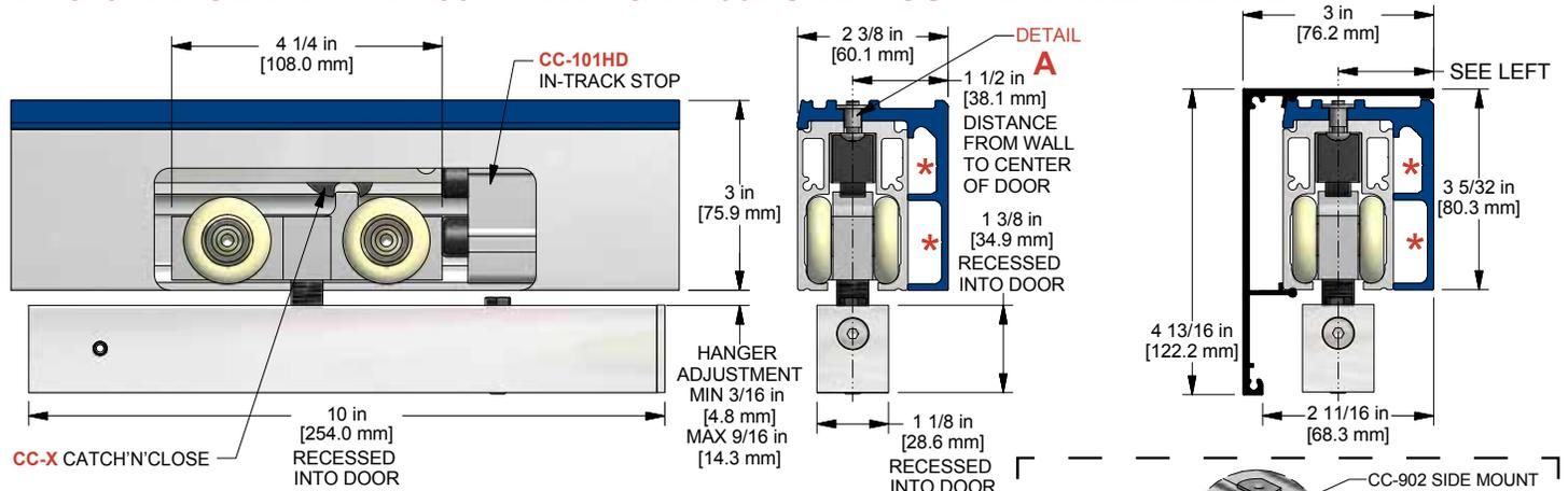
[CC-902 Side Mount Bracket illustrated as solid blue profile. Supplied in continuous lengths.]
