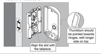
3g Secure the inside cover with two screws.
