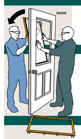
Once the screws are loosened, have a helper stand on the outside of the door and hold the frame. REMOVE ALL ATTACHMENT SCREWS AND REMOVE THE INNER FRAME.
