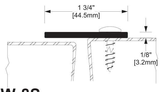
W-8S C.R. STEEL WITH CONDITIONED EDGES
