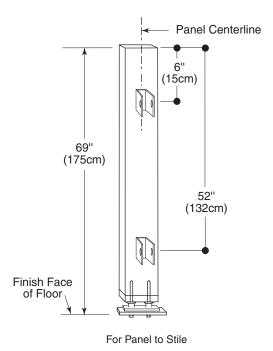
Fig. 5b: Overhead-Braced Bracket Placement.
