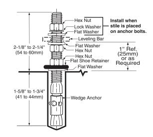
Fig. 2c: Detail of Ceiling Anchor.
