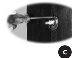
C. Secure adapter and plate with thrubolt screws making certain the lock washers are attached before tightening screws into thrubolt post of the outside rose assembly. **Do not over tighten.**
