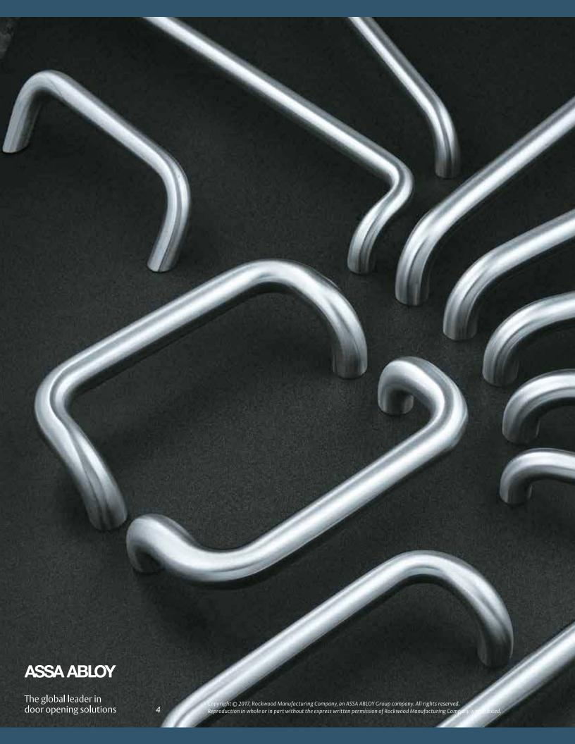
Our 11/4" and 11/2" diameter tubular pulls and pushes are made from rugged 16-gauge wall tubing with solid brass end inserts. These large diameter pulls provide a greater door contact area (11/4" pulls have 60% larger and 11/2" pulls have 125% larger mounting area) than 1" pulls, which ensures the fastening system will provide a tight, permanent installation. Our RM257 series is made from solid 11/4" rod and its 30° angle cut provides a mounting footprint 80% larger than 1" pulls.
