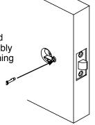
**Note:** Loosening the pre assembled #6-32 screws on the outside mounting plate may improve alignment for thicker doors.
