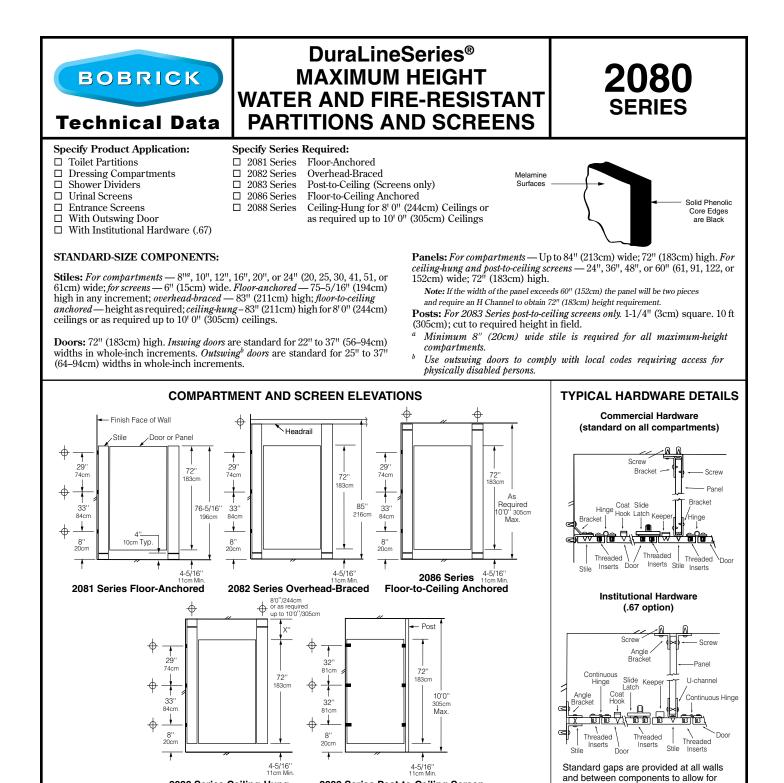
2088 Series Ceiling-Hung 2083 Series Post-to-Ceiling Screen + These mounting points require backing. For suggested backing methods, Bobrick Advisory Bulletins TB-32 for ceiling-hung installations and TB-46 for floor-anchored are available upon request
