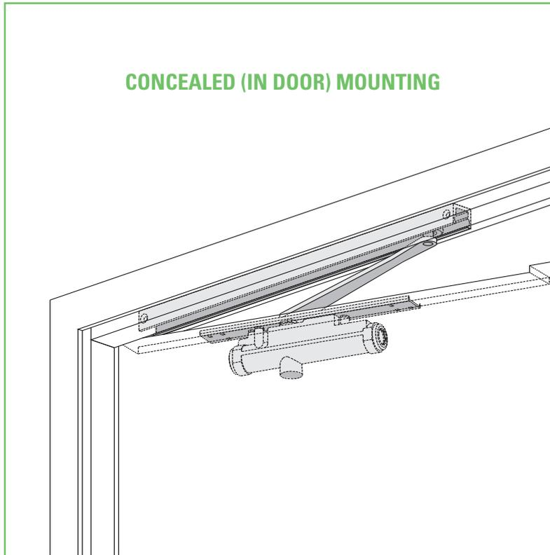
*The concealed 3130 is designed to mount in a 1 3/4" interior door. The single lever arm and roller assembly provides complete concealment and the choice of finishes and track functions meet virtually all architectural requirements.*
