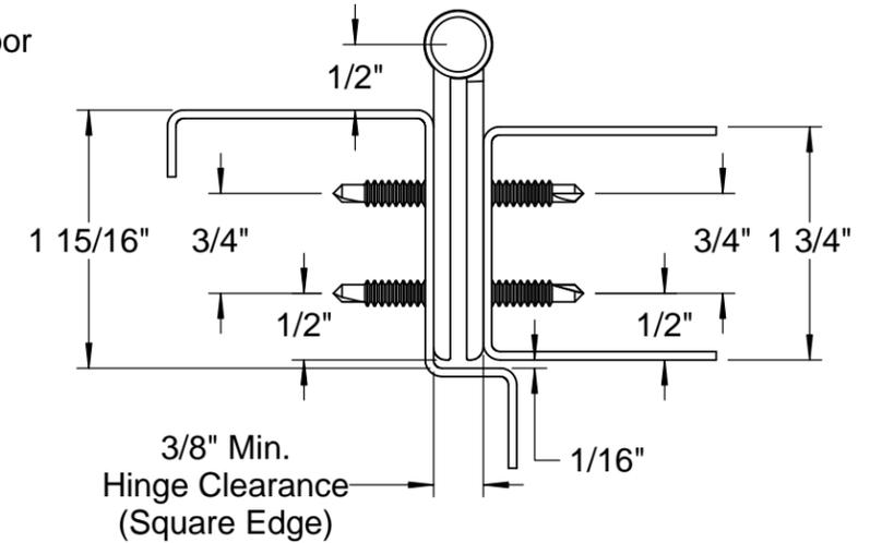
FIGURE 5: HINGE PLACEMENT & CLEARANCE TEMPLATE
